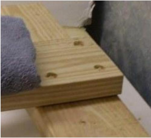
Counterbore the back holes on the top board and on the bottom side of the bottom board. This way the bolts will sit inside the wood and not stick out. Insert the 1/4 inch by 3 inch bolts through each hole and put a washer both top and bottom. No washers go between the boards. Screw these down tight and use a lock washer against the nut, and apply loctite if you have some. Make sure this is nice and tight and there are no sharp bolt edges sticking out anywhere.
