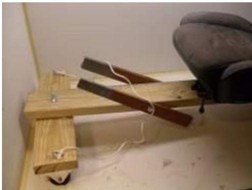
The brakes to lean forward as shown in the picture at left. This way they are easy to grab and they don't rub on the ground when you don't want them to. You do this by screwing a stop bolt near each brake. This is shown in the next picture
