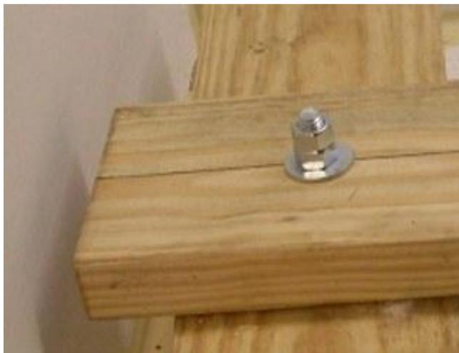
Install the big bolt in the front of the goKart. Do it this way. Insert it from the bottom with a washer between it and the bottom of the bottom board. Then insert two washers between the boards then insert one washer on the top. Finally put a nut on it and tighten it so it is tight but the board still smoothly moves as you would push it with your feet. Now install a second bolt and tighten it very tight against the first bolt. This allows it to stay tight without moving. With the nuts on
