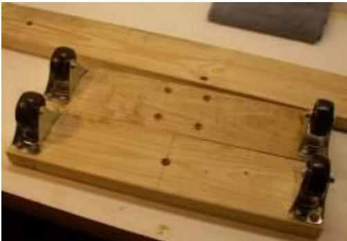
Optionally, you can attach the wheels to the 24 inch boards before you attach the boards to the main board. You can see here everything has been pre-drilled ready to assemble.
